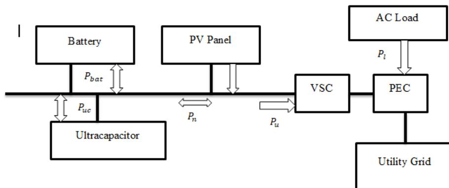
Figure 1. DC micro-grid system layout.
